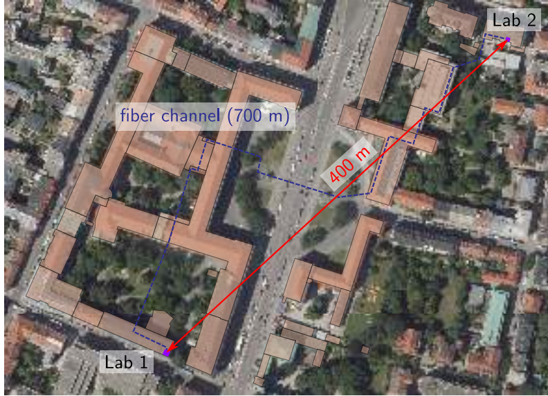
Figure 2.6.: Location of the two laboratories at the main campus of the Ludwig-Maximilians-Universität, Munich. Laboratory 1 (Lab 1) and Laboratory 2 (Lab 2) are located in the basement of the departments of the faculty of physics at Schellingstraße 4 and economics at Schackstraße 4. Optical fibers for communication and for guiding the fluorescence photons emitted by the atoms are connecting the two laboratories. Map data provided by the Bayerisches Landesamt fuer Digitalisierung, Breitband und Vermessung.
