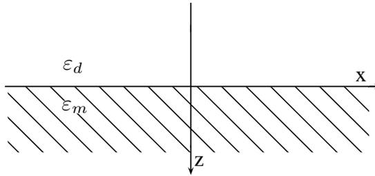
Figure 2.1.: Plane interface of a dielectric and a metallic conductor.
