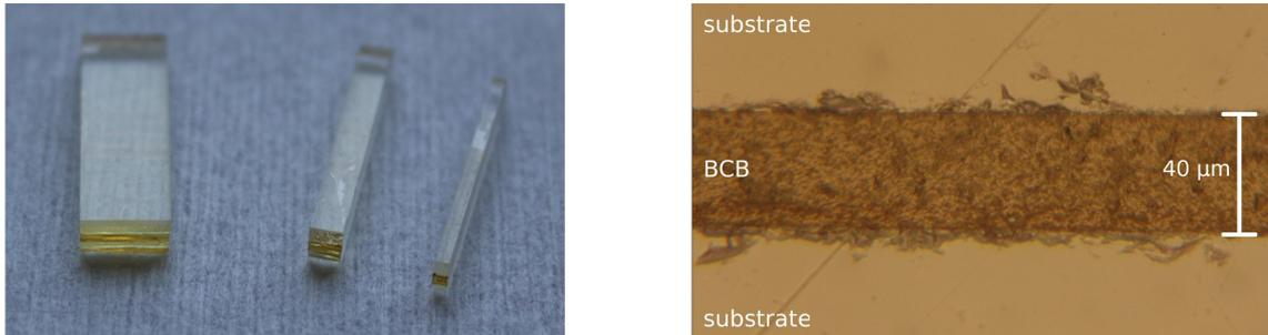
Figure 4.8.: Left: Wave guides of 5, 2 and 1 mm length (from left to right), Right: Microscope picture of a polished wave guide facet
