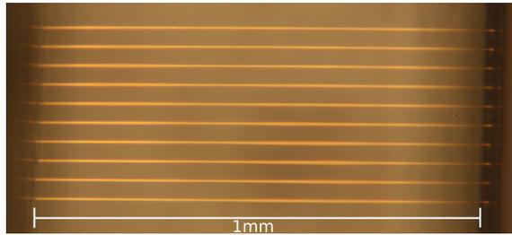
Figure 4.9.: Microscope picture of a finished wave guide. The stripes seen have a designed width of  $4\ \mu\text{m}$ .
