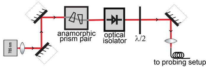
Figure 5.1.: Schematic sketch of the setup's section that is used to create a well defined light mode
