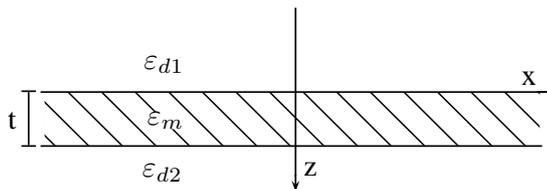
Figure 2.3.: Double interface of a dielectric-metal-dielectric sandwich structure
