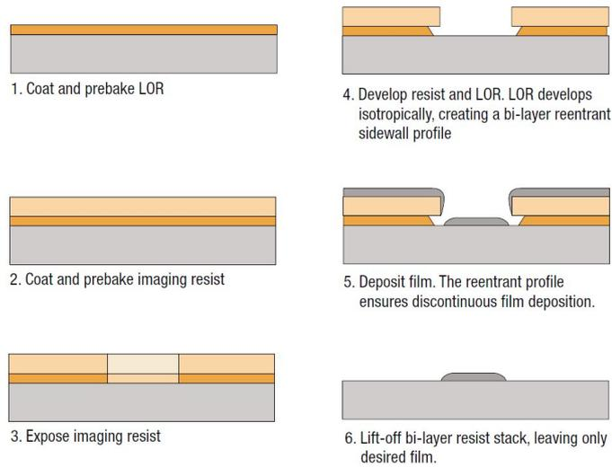
Figure 4.1.: Process steps for photolithography with a sacrificial layer (LOR) in order to create an undercut [20].
