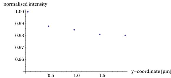
Figure 5.7.: Plot of the normalised intensity at the brightest spot for different distances between fibre end and wave guide facet. [gold stripe dimensions: thickness  $t = 17$  nm, width  $w = 5$   $\mu\text{m}$ , length  $l = 3$  mm]
