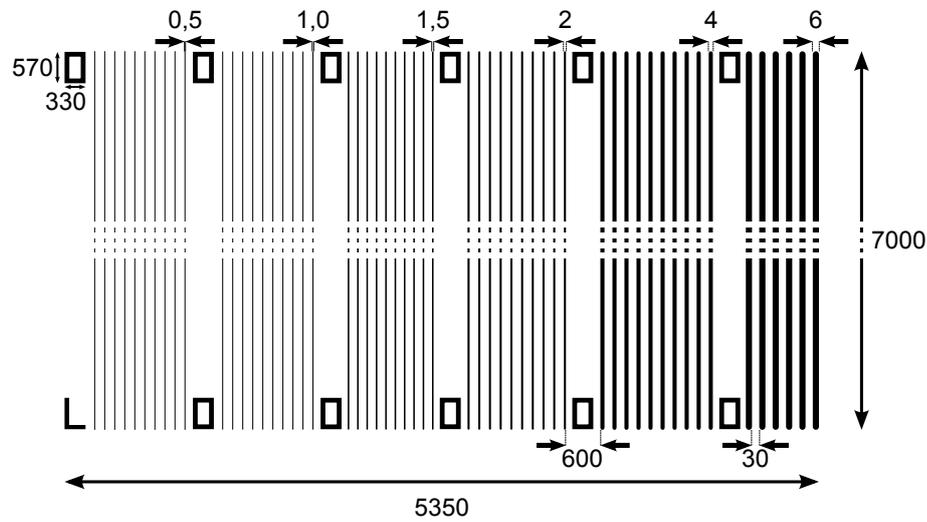
Figure 3.3.: Schematic sketch of the photomask and with that the gold pattern of the wave guide
