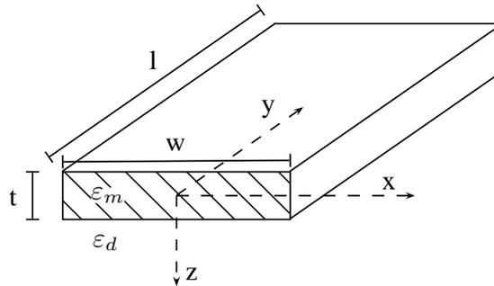
Figure 2.6.: Schematic of a metal stripe surrounded by a dielectric used for long-range surface plasmon polariton propagation. Propagation direction is the  $y$ -direction.
