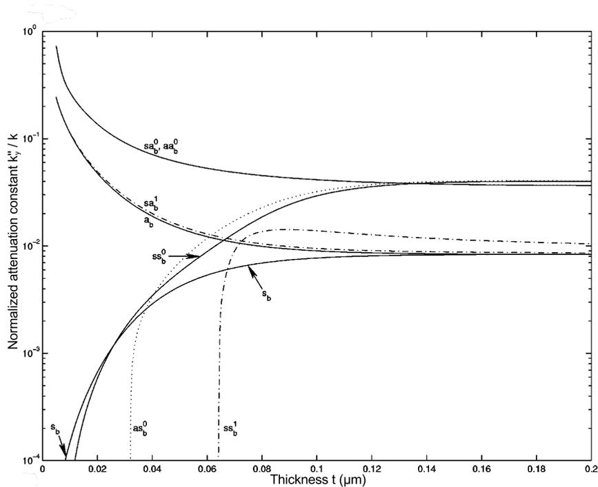
Figure 2.7.: Normalised attenuation constant versus metal thickness  $t$  with stripe width  $w = 0,5 \mu\text{m}$ . In addition to the four fundamental modes in the gold stripe, the first higher order modes  $sa_b^1$  and  $ss_b^1$  are shown, as well as the s- and a-mode of the infinite metal film (denoted  $s_b$  and  $a_b$  here). Adapted from [8].
