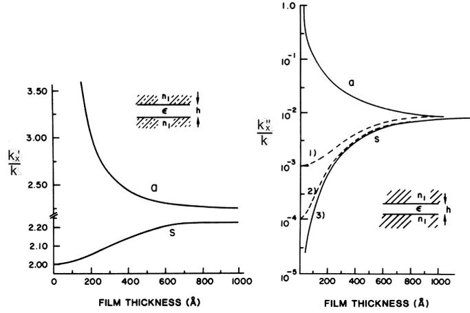
Figure 2.5.: Normalized complex propagation wave vector  $k_y/k$  as a function of the film thickness for the symmetric structure with  $\sqrt{\epsilon_1} = 2.0$ .  $a$  and  $s$  refer to the asymmetric and symmetric mode, respectively. (1)  $\sqrt{\epsilon_1} = 2.0 - 0.001 i$ , (2)  $\sqrt{\epsilon_1} = 2.0 - 0.0001 i$ , and (3)  $\sqrt{\epsilon_1} = 2.0$ ,  $\epsilon_m = -19 - 0.53 i$ . Adapted from [15].
