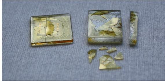
Figure A.3.: Two dies, each with a cracked BCB layer that has been destroyed during sawing
