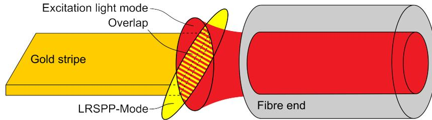
Figure 5.5.: Schematic sketch of the overlap measurement. The overlap of the excitation light mode (red) and of the LRSPP mode (yellow) is illustrated as the hatched area.
