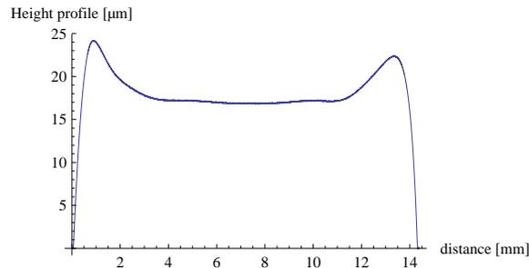
Figure A.1.: Profile of the BCB layer with edge bead after soft cure
