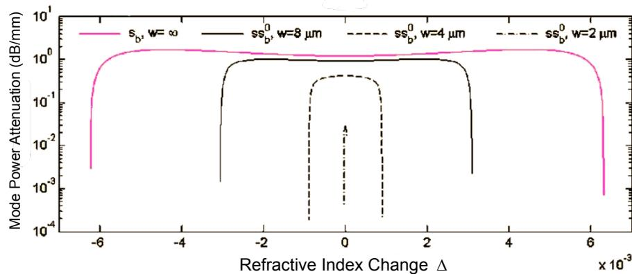
Figure 3.1.: Mode power attenuation as a function of the refractive index asymmetry  $\Delta$  for various stripe widths with thickness  $t = 20$  nm.  $\varepsilon_{d1} = 1,447$ . Adapted from [19].
