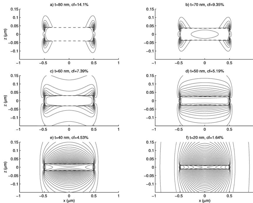
Figure 2.8.: Contour plot of the real part of the Poynting vector  $S_y$  associated with the  $ss_b^0$  mode for metal films of width  $w = 1 \mu\text{m}$  and various thicknesses. The outline of the stripe's cross-section is shown as the rectangular dashed contour. Adapted from [8].
