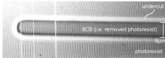
Figure 4.3.: Microscope picture of the photoresist and lift-off resist after development. The undercut shows as a bright margin around the stripe. (designed stripe width:  $6\mu\text{m}$ )
