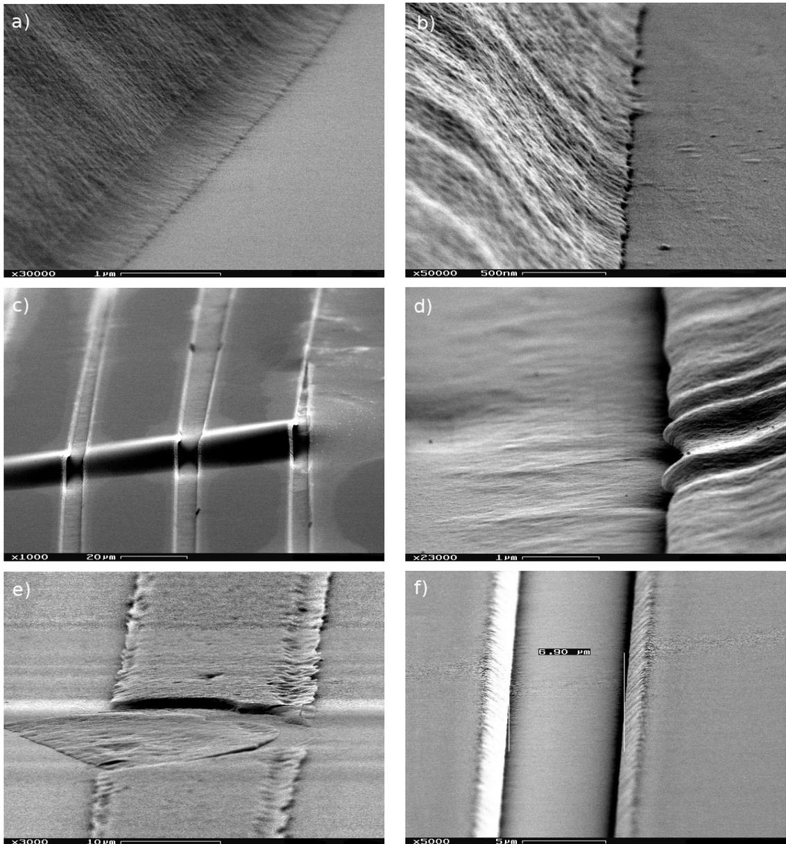
Figure A.2.: Scanning electron microscope pictures of different attempts to create an undercut in the resist structure
