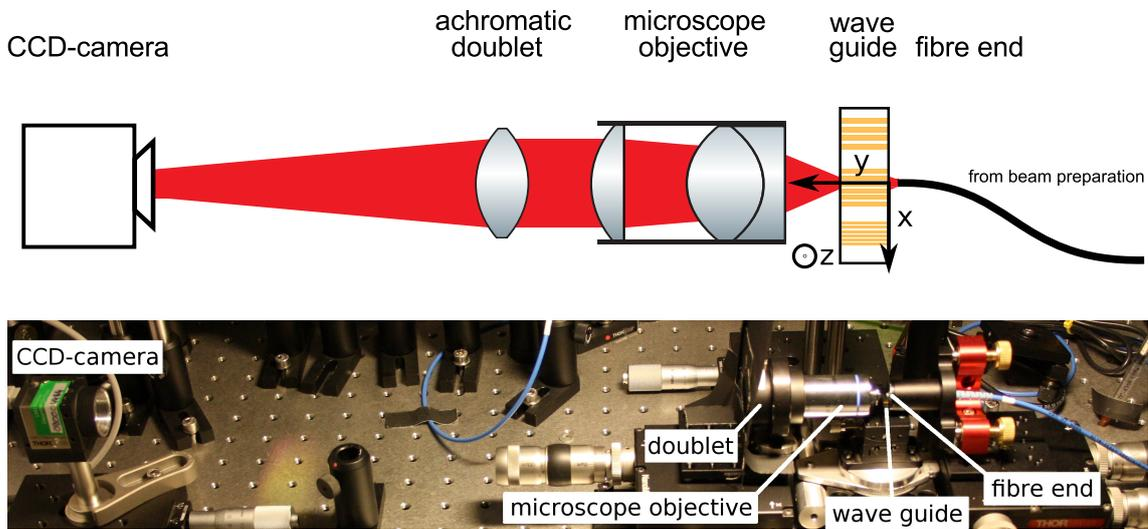
Figure 5.2.: Schematic sketch (top) and photograph (bottom) of the probing part of the setup. The arrangement of the fibre end, wave guide and microscope objective can be seen on the right, the CCD-camera on the left.
