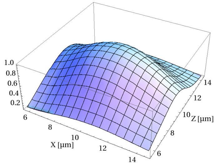
Figure 5.6.: Measured overlap of a Gaussian optical mode from the fibre with the LRSPP mode. The center of the gold stripes cross-section lies at  $x = 10 \mu\text{m}$ ,  $y = 10 \mu\text{m}$ . [gold stripe dimensions: thickness  $t = 17 \text{ nm}$ , width  $w = 5 \mu\text{m}$ , length  $l = 3 \text{ mm}$ ]
