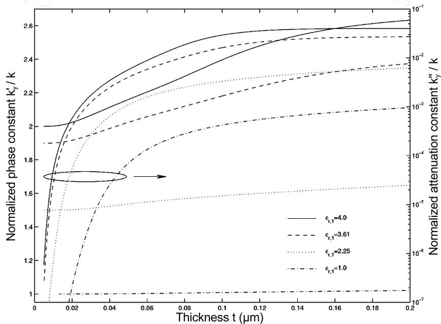
Figure 2.9.: Normalised propagation  $k'_y/k$  and normalised attenuation constant  $k''_y/k$  as a function of the metal thickness  $t$  ( $w = 0,5 \mu\text{m}$ ) for various permittivities of the metal surrounding dielectric  $\epsilon_d$  (in the plot  $\epsilon_{r,1}$ ). The normalized phase constant is plotted on the left axis and the normalized attenuation constant is plotted on the right one. Adapted from [8].
