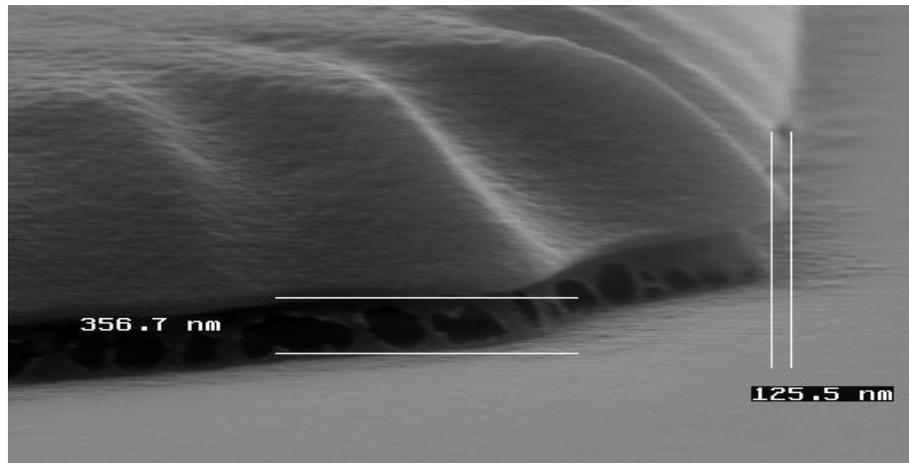
Figure 4.4.: Picture of an undercut taken with a scanning electron microscope at a magnification of 19500x.
