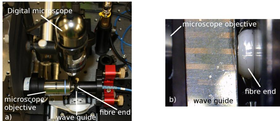
Figure 5.3.: a) Photograph of the fibre end, wave guide and microscope objective arrangement and the digital microscope. b) Picture of the digital microscope taken during alignment.
