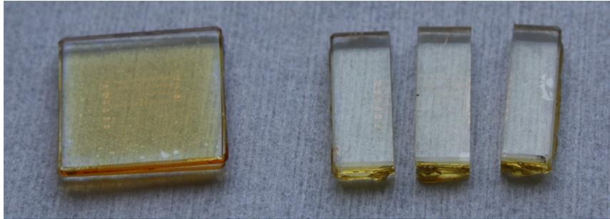
Figure 4.7.: Two dies, the left one before the right one after sawing.
