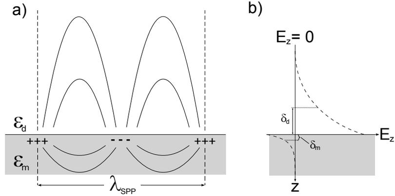
Figure 2.2.: Schematic sketch of the metal-dielectric interface. Both drawings illustrate that the majority of the electric field is located in the dielectric medium a) Electric field and charge distribution at the interface. b)  $z$ -component of the electric field in dependence of the distance to the interface.
