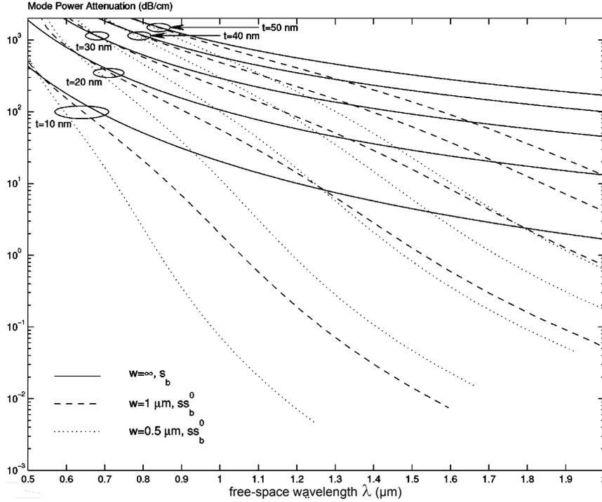
Figure 2.10.: Calculated Mode Power Attenuation in dB/cm of the  $ss_b^0$  mode in dependence of the free space wavelength of the incident light. Metal stripe width  $w = 0.5 \mu\text{m}$  and  $w = 1 \mu\text{m}$  and various thicknesses  $t$ . The s-mode supported for the case  $w = \infty$  is shown for comparison (solid lines). Adapted from [8].
