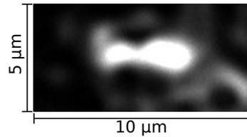
Figure 5.4.: Microscope picture of the plasmon mode at the end facet of the wave guide. [gold stripe dimensions: thickness  $t = 17$  nm, width  $w = 5$   $\mu\text{m}$ , length  $l = 3$  mm]
