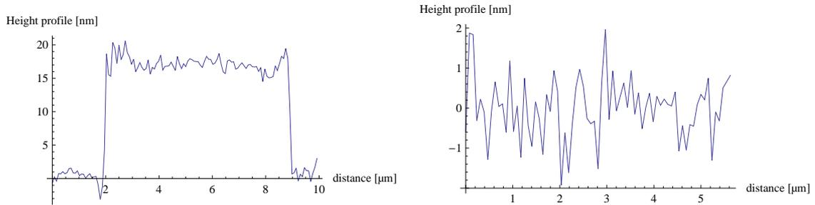
Figure 4.6.: Width and height of the gold stripe measured after lift-off with an AFM after lift-off. Left: profile of the gold stripe Right: roughness of the gold stripes' surface. The designed width of the stripe is 4  $\mu\text{m}$
