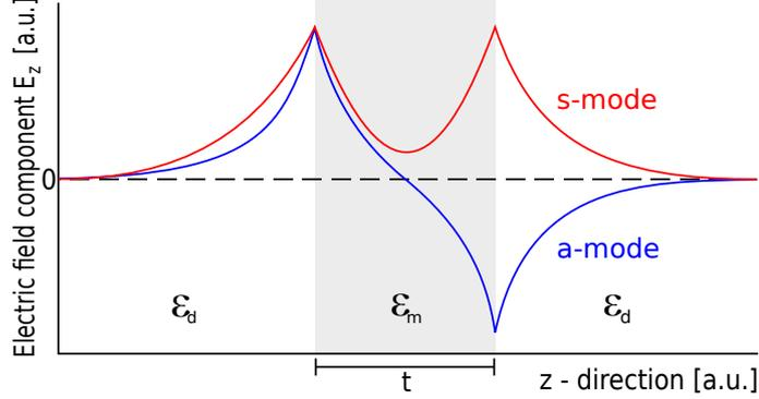
Figure 2.4.: Sketch of the amplitude of the  $E_z$  field component across a thin metal film. The surface plasmon polariton forms two modes, one with a symmetric (s-mode) and one with an asymmetric (a-mode) field distribution inside the metal film [15].
