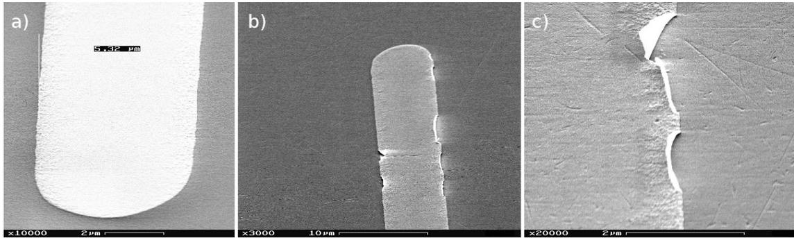
Figure 4.5.: Scanning electron microscope picture of gold stripes after the lift-off. (a) stripe with good edge quality (b),(c) stripes with lower edge quality. The gold layer lifted at the edges due to poor lift-off.
