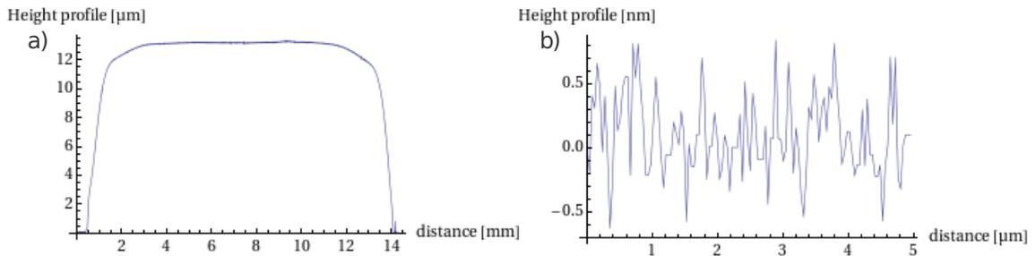
Figure 4.2.: Profiles of the lower layer of BCB with removed edge bead and after soft cure, a) Profile over the entire substrate b) Roughness of the surface, taken with an AFM
