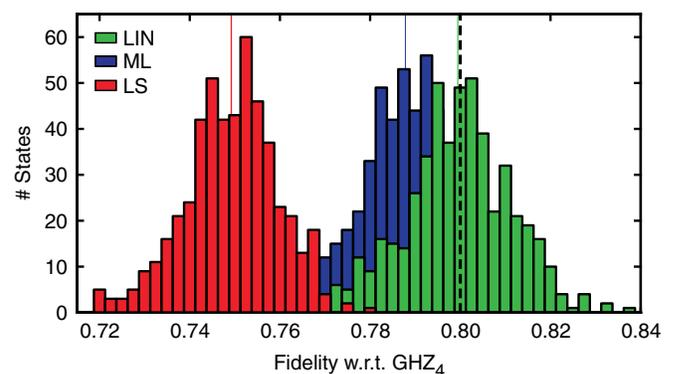
FIG. 1 (color online). Histogram of the fidelity estimates of 500 independent simulations of QST of a noisy four-party GHZ state for three different reconstruction schemes. The values obtained via ML (blue) or LS (red) fluctuate around a value that is lower than the initial fidelity of 80% (dashed line). For comparison, we also show the result using LIN (green), which does not have this systematic error called bias.
