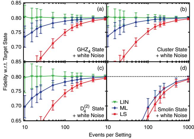
FIG. 2 (color online). The performance of ML, LS, and LIN methods depending on the number of events  $N_s$  per setting and for four different noisy initial states  $\rho_0$ . Note that the fidelity can only be calculated linearly if the reference state is pure which is not the case for the Smolin state [25]. Therefore, only the curves for ML and LS are plotted for the Smolin state.
