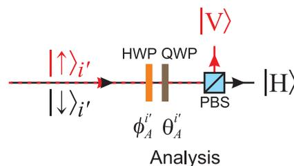
FIG. 9. (Color online) If Alice wants to measure in the basis  $\sigma_{i'} = |\downarrow\rangle_{i'}\langle\downarrow|_{i'} - |\uparrow\rangle_{i'}\langle\uparrow|_{i'}$  ( $i = x, y, z$ ), then the HWP and the QWP of the polarization analysis have to be aligned such that  $|\downarrow\rangle_{i'}$  and  $|\uparrow\rangle_{i'}$  are detected at different outputs of the PBS. The same holds for Bob.
