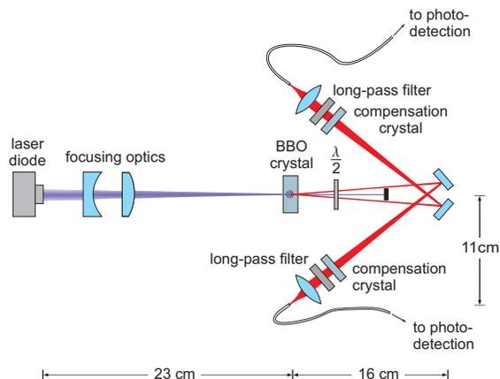
Fig. 1. Schematic set-up of the source. The single-mode cw laser diode operating at 402.6 nm pumps a 2 mm thick BBO crystal and produces polarization-entangled photon pairs at 805.2 nm collected into single-mode fibres. For compensation of the walk-off, two additional BBO crystals preceded by a half-wave retarder are used.
