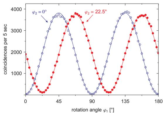
Fig. 4. Polarization correlations between photons of a pair measured in the H/V (-o-) and  $+45^\circ / -45^\circ$  (-●-) polarization basis. The visibilities obtained from a  $\sin^2$  fit (solid lines) to the measured coincidence count rates are  $98.3 \pm 0.1\%$  and  $94.3 \pm 0.2\%$ , respectively.
