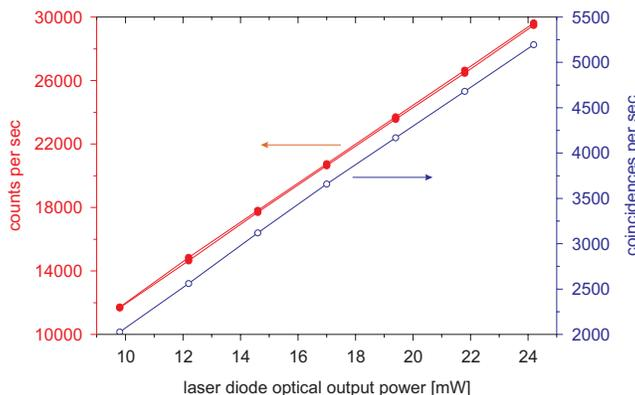
Fig. 2. Single (●) and coincidence (○) count rates depending on the pump power measured right behind the violet laser diode.
