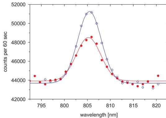
Fig. 3. Spectral distributions of the down-converted light collected into single-mode fibres. Both photons of the pair have nearly the same wavelength with separation only 0.22 nm around the degeneracy wavelength of 805.2 nm. The least-square Gaussian fit (solid lines) to measured data points shows FWHMs of  $6.03 \pm 0.14$  nm (-o-) and  $6.24 \pm 0.56$  nm (-●-), respectively. The offset of 44000 counts is due to the dark counts of the Si APDs.
