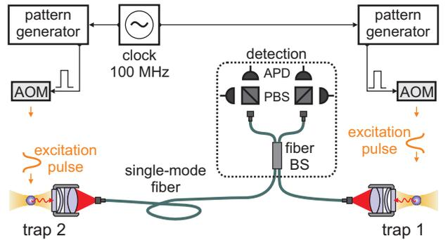
Figure 2: Two synchronized atomic traps located in separate laboratories. The optical excitation pulses are shaped by acousto-optic modulators (AOMs) such, that the emitted photons arrive simultaneously at the fiber beam splitter (BS) for interference. The timing is controlled by two electronic pattern generators driven by a common clock. The photons leaving the beam splitter are detected by avalanche photodiodes (APDs) after their polarization was analyzed by polarizing beam splitters (PBS).
