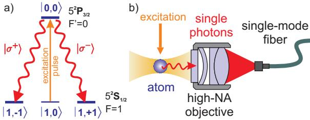
Figure 1: a) Principle of generation of single photons whose polarization is entangled with the atomic spin. b) The emitted photons are collected by an objective and coupled into a single-mode optical fiber for interference experiments.
