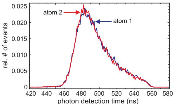
Figure 3: Histograms of the arrival time of single photons emitted by two optically trapped atoms after passing a fiber beam splitter. The arrival times were measured independently with respect to a common clock. Both histograms are individually normalized with respect to the total number of events.
