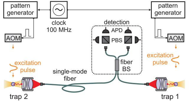
Figure 2: Two synchronized atomic traps located in separate laboratories. The optical excitation pulses are shaped by acousto-optic modulators (AOMs) such, that the emitted photons arrive simultaneously at the fiber beam splitter (BS) for interference. The timing is controlled by two electronic pattern generators driven by a common clock. The photons leaving the beam splitter are detected by avalanche photodetectors (APDs) after their polarization was analyzed by polarizing beam splitters (PBS).
