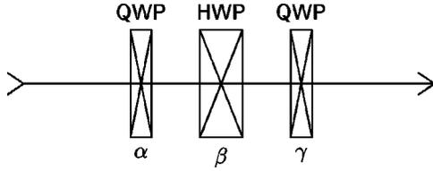
FIG. 2. By sending a photon through a QWP, then through a HWP, finally through another QWP, its polarization state can be changed unitarily to any other one.
