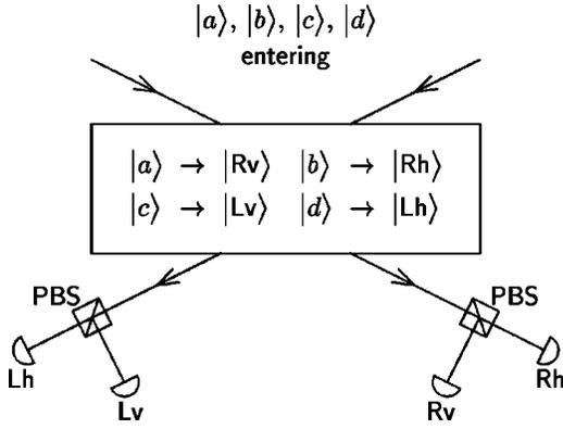
FIG. 5. For a measurement of an arbitrary 2-qubit basis, consisting of the mutually orthogonal states  $|a\rangle$ ,  $|b\rangle$ ,  $|c\rangle$ , and  $|d\rangle$ , one first transforms it to the standard basis with the aid of an appropriate 2-qubit gate. The output is sent through PBS's that reflect vertically polarized photons and transmit horizontally polarized ones. A click of either one of the four photon detectors (symbolized by semi-circles) is indicative of the respective input state.
